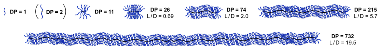
Figure 4. Schematic of the bottlebrush polymers, aPP-NB macromonomer, and hypothetical “dimer” with backbone DP = 2. Length to diameter aspect ratios ( L/D ) are given for the highest molecular weight bottlebrushes assuming fully extended polymer chains.
